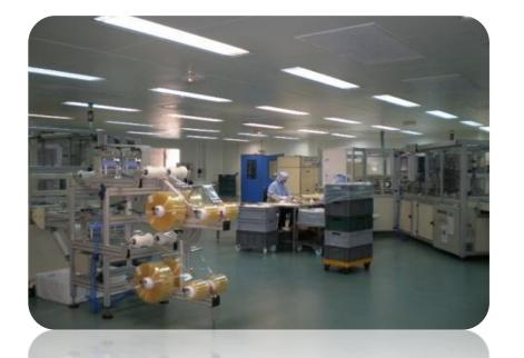
Manufacturing environment needs to be controlled to prevent contamination of bags :
