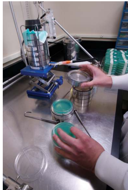
Bacterial Filtration Efficiency Testing
