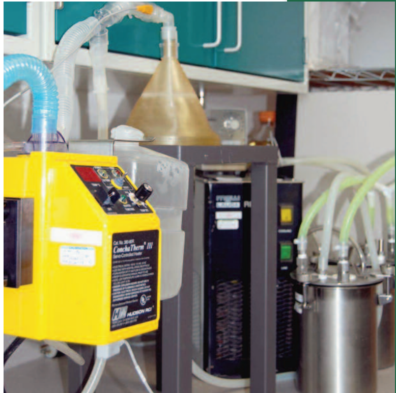
Collection of antimicrobial particles using simulated inhalation setup.
